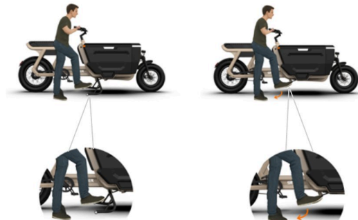
Figure 6 • Lowering the centre stand
